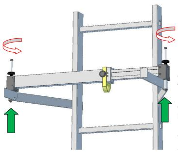
After adjustment, the U/S-WEA Universal Attachment Point is now clamped to the ladder brackets by turning the star handles of the relevant clamping device. The clamping lugs must surround the bottom side of the vertical ladder mount, in order to securely tighten the U/S-WEA Universal Attachment Point.
