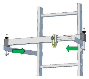
Both clamping devices are now pushed towards the middle, until they make contact with the ladder brackets. The contact surfaces must now lie on the ladder bracket.
