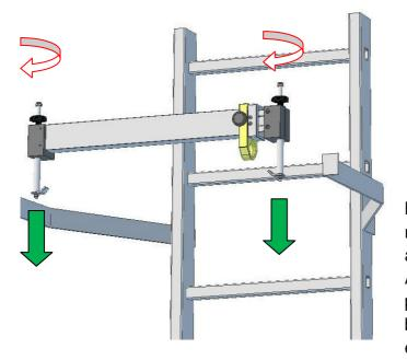
An approved and tested safety harness with a restraining system must be used for installation and assembly. The U/S-WEA Universal Attachment Point must be positioned above the ladder bracket with the clamping device extended.
